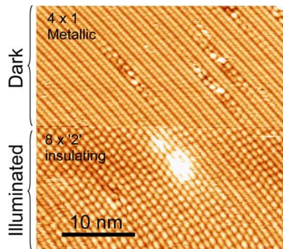
Fig. 1. Optical control of transition from  $4 \times 1$  metallic (upper area) to  $8 \times 2$  insulating (lower area) phases.
